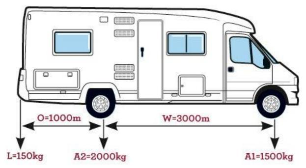
A1 = existing front axle load (before adding on the new rear load)
